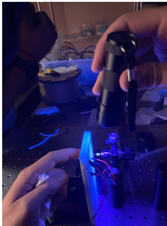
Figure 6.1-4. UV Flashlight Curing UV Resin
