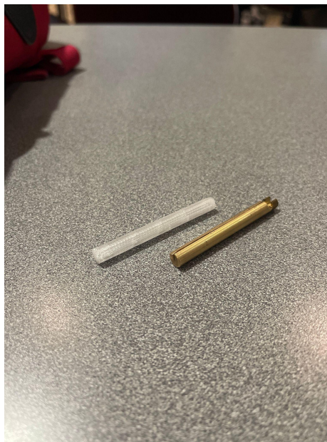
Figure 4.8.2-2. 3D Printed Side Loaded Fiber Chuck
