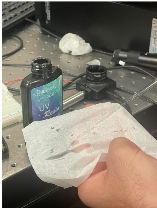
Figure 3.3.4-1. UV Resin To Seal LED-Fiber Coupling
