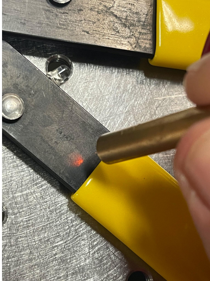
Figure 6.1.2-1 Spatially Coherent Light Exiting Fiber as a Point Source
